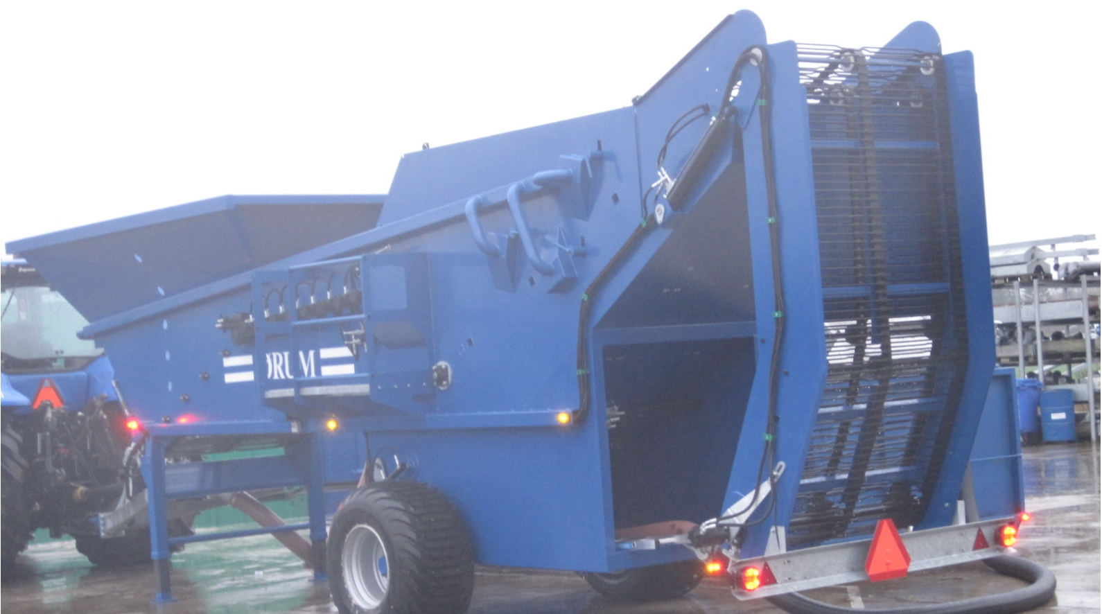
Elevator i transportstilling.
